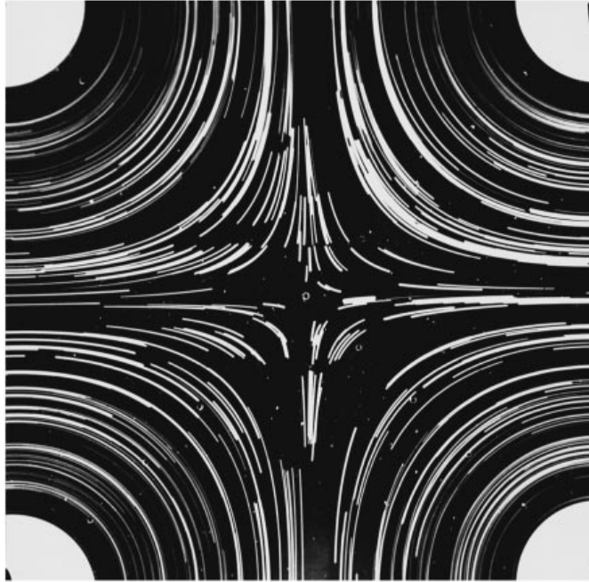
FIGURE 2. Photograph showing the trajectories of the tracer particles in the mid-plane of the tank, 4 h after the start of the forcing. The flow was generated by four rotating horizontal discs, and the strain rate e near the centre of the tank was 0.80 \times 10^{-2} \text{ s}^{-1} . The photograph was taken with an exposure time of 120 s. Experimental parameters: \Omega_d = 3.0 \text{ r.p.m.} , D = 50 \text{ cm} and N = 2.8 \text{ rad s}^{-1} .
